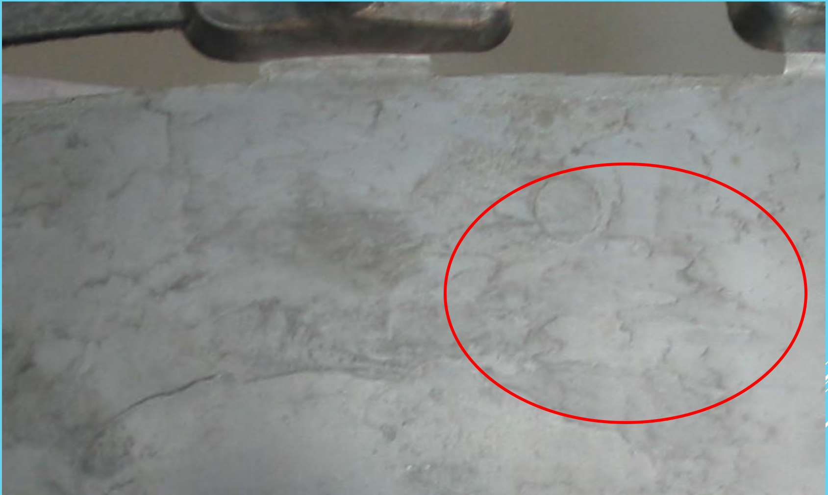
stained casting(油污,油纹)
