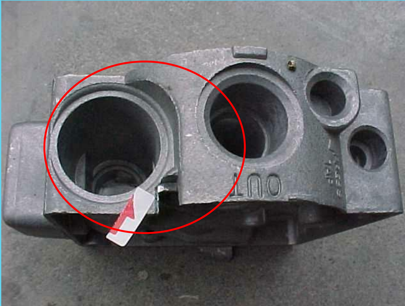
mold collapse (崩模)
